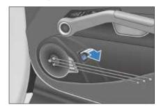
When the trunk is open and the switch is pulled for more than one second, the lid closes automatically. Release the switch to freeze the closing motion.
