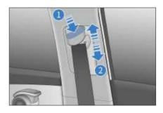
5. Pull the belt firmly to check that the adjuster is locked.
