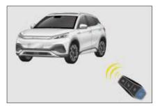
3. After the vehicle is started, pressing and holding the remote start/stop button on the smart key for two seconds switches the ignition off. The turn signals then flash twice.
