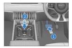
The vehicle is ready to drive when the OK indicator lights up on the instrument cluster.
