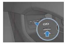
The driving recorder supports TF card (also called Micro-SD card) from 64 to 128 GB with a Class 10 speed rating or higher.
