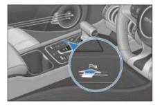
When the parking assist system is enabled, the vehicle is not in "P", and the Electronic Parking Brake (EPB) and Auto Vehicle Hold (AVH) are released, the obstacle detection mode of the parking assist system is enabled. When enabled, the system raises an alarm if obstacles are found surrounding the vehicle; when disabled, it does not.
