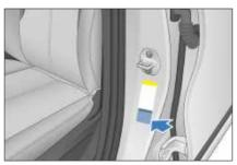
The child protection lock label is engraved on the metal sheet surface on the left/right rear door.
