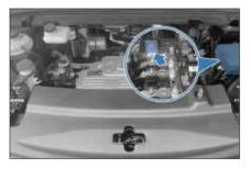
Negative terminal for jump starting: Unpainted metal on the motor assembly such as bolts as shown.
