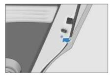
The charging connector use tip label is attached to the inner surface of the charge port door.
