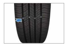
Tires with exposed wear bars are experiencing serious performance loss and therefore must be replaced.
