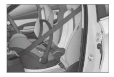
ISOFix/i-Size anchorage points are available for the front passenger seat and the label indicating an anchorage point location is attached to the seatback above the relevant anchorage  An anchorage is provided for child restraint installation at the back of the front passenger seat.
