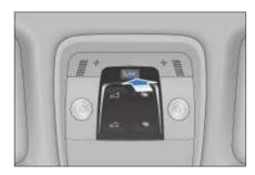
The E-Call system activates automatically in the event of airbag deployment or the detection of a severe collision.
