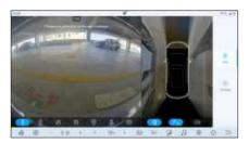
After the vehicle starts, the image before last power-off is displayed on the transparent panoramic view screen. Foreign bodies shown may be inconsistent with the actual ones in the underbody and surrounding blind areas. The underbody image update will begin only after the vehicle has started to run and will be complete when the vehicle has been driven beyond its length.
