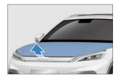
3. After closing the hood, check whether the latch is securely locked. If the hood can be lifted slightly, it indicates that it is not properly locked. Open the hood again and then close it correctly according to the above steps.
