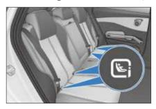
Rear outboard seats are equipped with tether strap anchorages on the back. Middle seat anchorage depends on configuration.  The use of top tether anchorage point with a belted child restraint is allowed in specific markets only.
