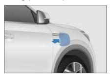
· Open the charge port cap and the protective cover\* of the charging connector, and make sure that no
